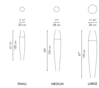
Surface mounted pre-wired lamp E26 / E27 110V - 230V
